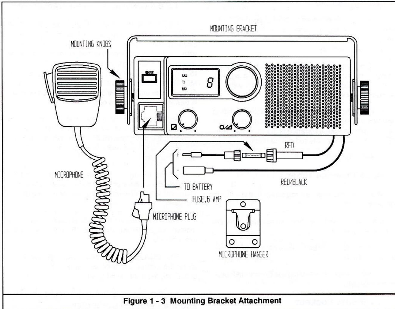
Figure 1 - 3 Mounting Bracket Attachment
