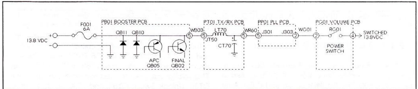
Figure 2-1 Unswitched +13.8VDC Power Distribution
