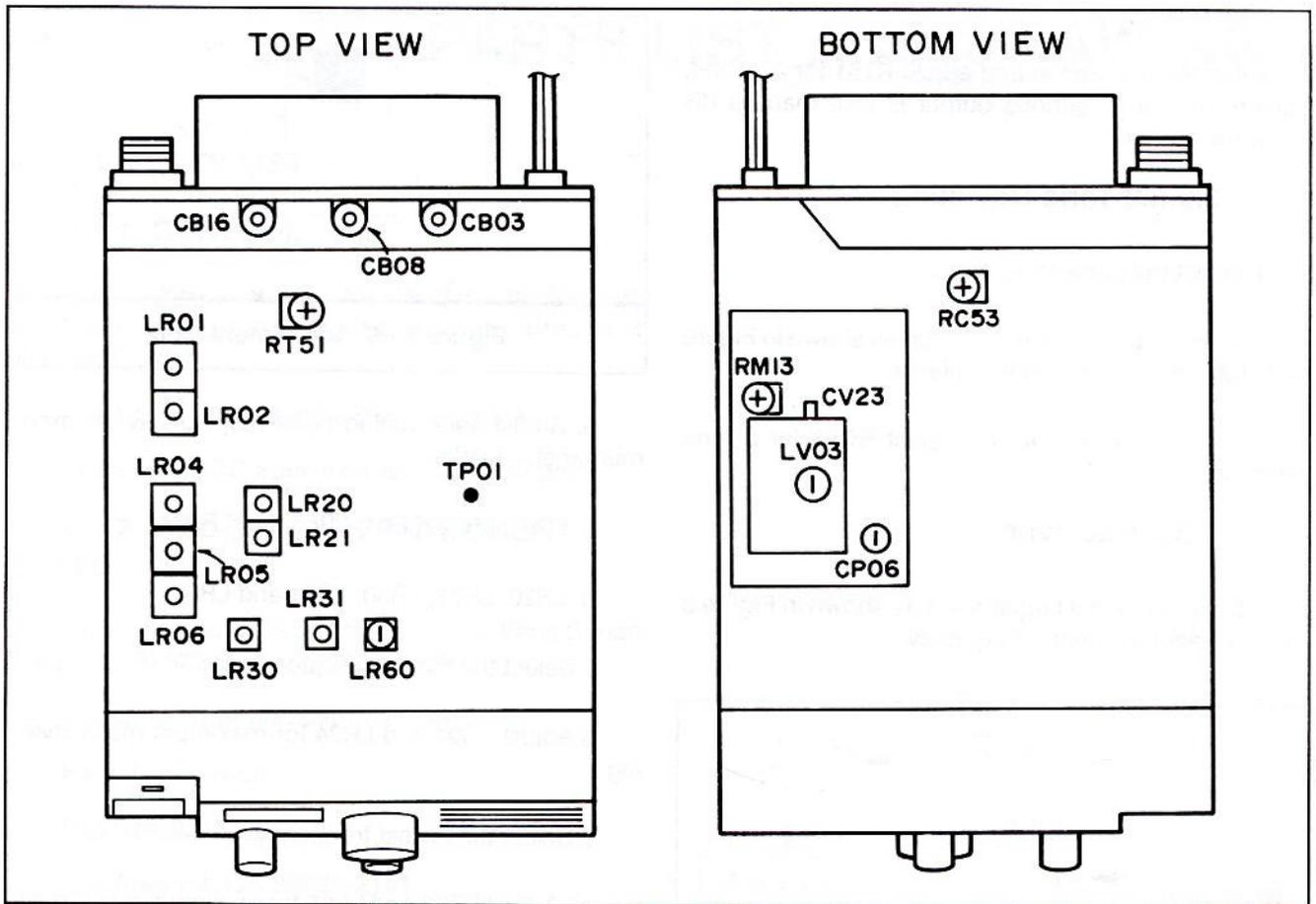
Figure 3 - 2 Alignment Reference Points
