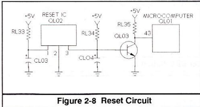
**Figure 2-8 Reset Circuit**
