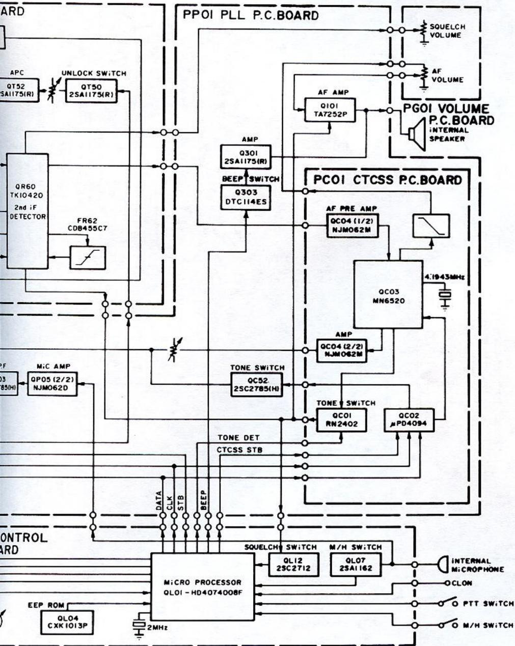
Figure 4-1 GX1500V Functional Block Diagram
