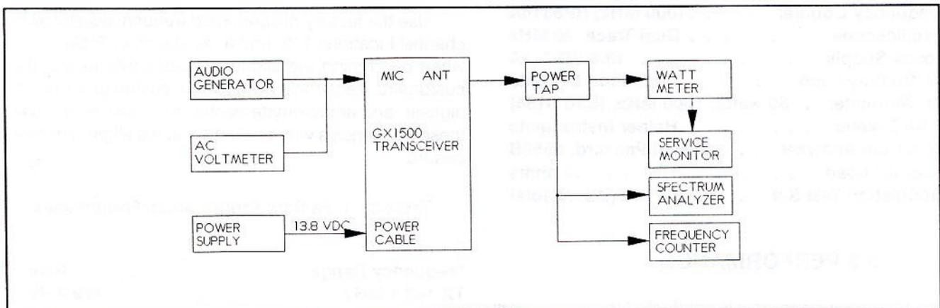
**Figure 3 - 1 Equipment Test Setup**
