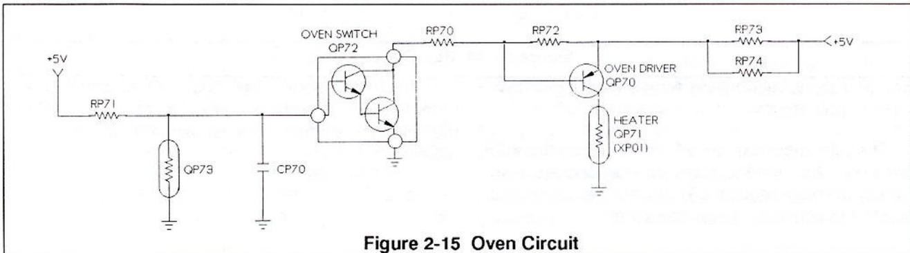
Figure 2-15 Oven Circuit
