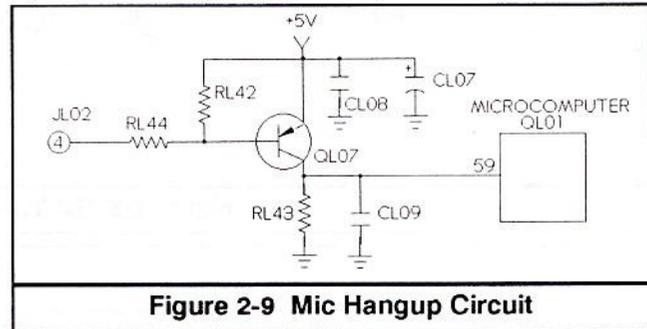
**Figure 2-9 Mic Hangup Circuit**
