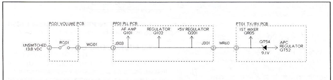
Figure 2-2 Switched +13.8VDC Power Distribution
