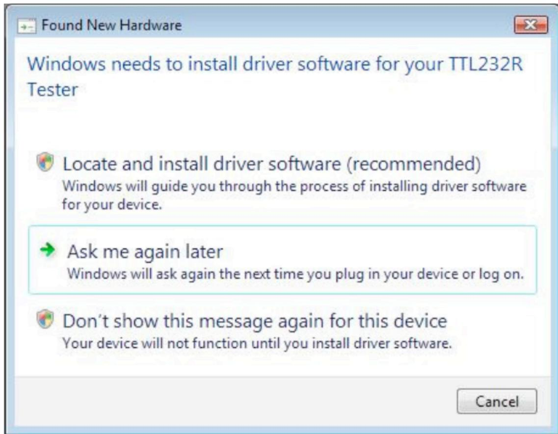
When "Locate and install driver software (recommended)" is selected the following screen will appear.
