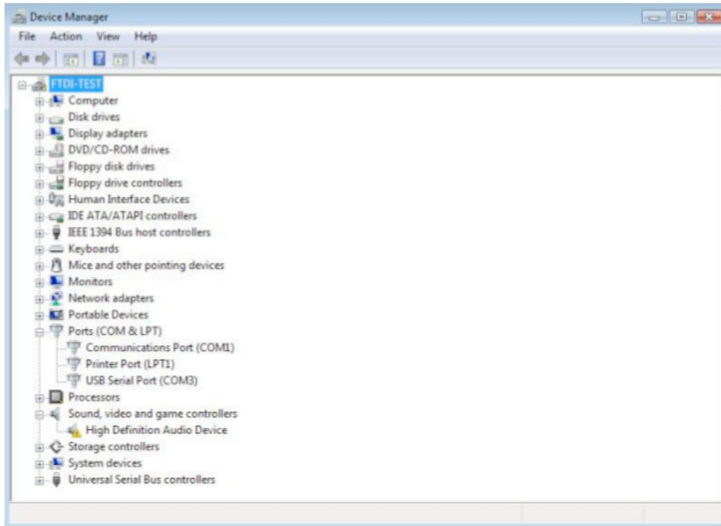
This screen shows the device connected to COM3. It may be different on your computer. Whatever COM port is showing is the COM port that you will set your Minitor Programming software setting to.
